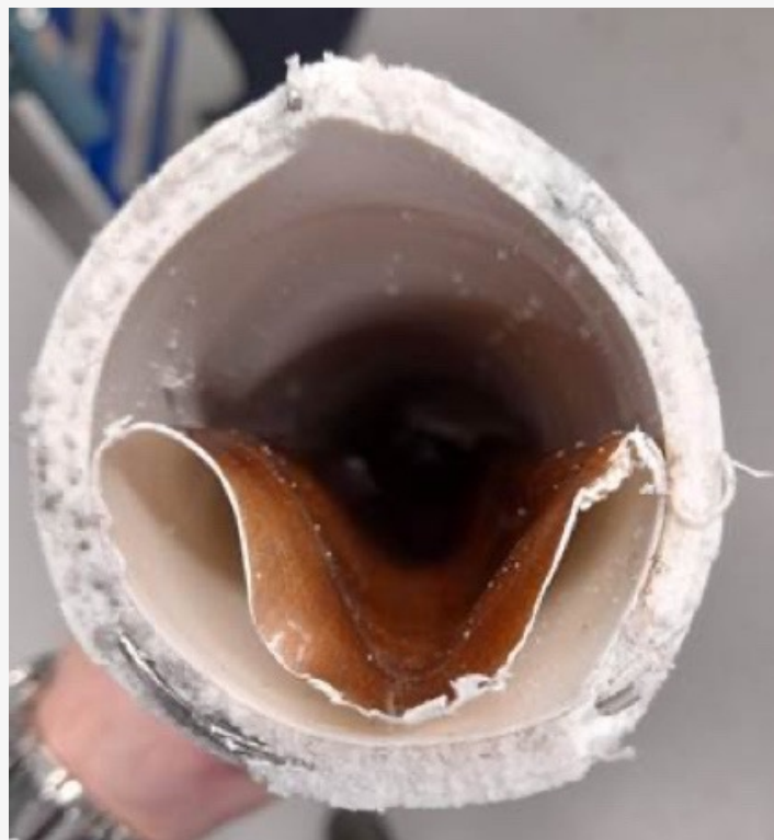
Figure: PTFE liner detached from hose cover
