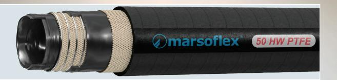
The marsoflex universal chemical hose type 50HW PTFE is a universally usable elastomer hose with a seamless, conductive inner layer made of black PTFE. Suitable for use in chemical, pharmaceutical and food industries.
